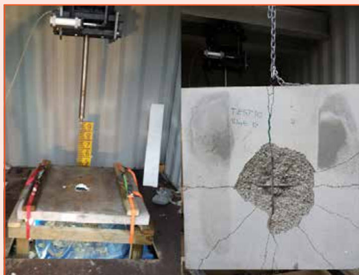
Impacts to reinforced concrete slabs. Left photo illustrating a full perforation with ~4 kg of concrete fragments ejected from the backface. Right illustrating the shear cone on the backface of a 1m by 1m slab post-impact. Photo credit: George Daly
